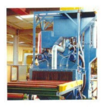
Sandstorm 4 Wheel Plate and Section De-Scalers have the capacity to process a wide range of types and sizes of steel and rolled or fabricated steel sections.
