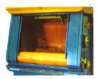
For applications with high sand loadings, such as foundary core knockout, double lip airwash separators are available, along with surge bins and by-pass systems, which continue to clean the abrasive even when the machine is in idle mode.
