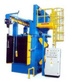
The Sandstorm Airless blast machines are designed to blast a large range of products while suspended and rotated on a hook arrangement.
